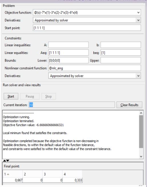
**EX11** Consider a firm and 3 inputs (X,Y,Z) in the production process. Consider the following production function depending on the quantities used of each input: f(x,y,z)=xy+yz. The unitary cost of each input is respectively 3, 10, 80. For the production at least two units of the third input must be used. The firm wants to maximize the production by having at most a total cost equal to 300.
