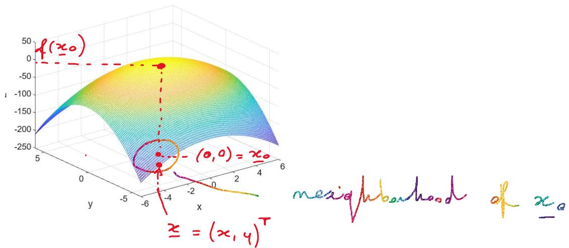
$$f(\underline{x}) - f(\underline{x}_0) \approx \frac{1}{2} \underbrace{\underline{h}^T \underline{\underline{H}} f(\underline{x}_0) \underline{h}}$$
